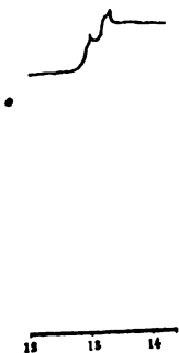
Fig. 1. Portion of Curve on 5-2-02 Showing the Slip of Fibre No. 3 Mounted in Instrument No. 1.
